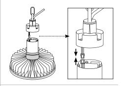
4. Align Fixture head's screw holes and firmly place. Note: there is only one correct aligned orientation.
