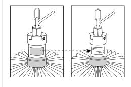
7. Pull the Fixture through the bottom of the reflector up until the reflector plate snaps into the slot of the black rubber ring.
