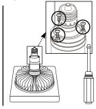
2. Detach lamp head and disconnect black electrical connector. Remove safety cable.
