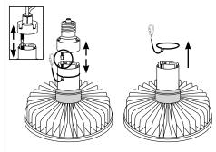
3. Attach the Fixture head's black electrical connector. Make sure the white markings are aligned.
