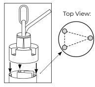
5. Place one of the screws through the safety hook adapter and into one of the three V3M holes. Insert the other screws into the remaining holes and screw in.
